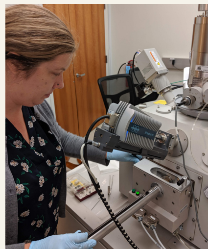
Jennifer Cooper analyzes biochar surface characteristics using scanning electron microscopy.
