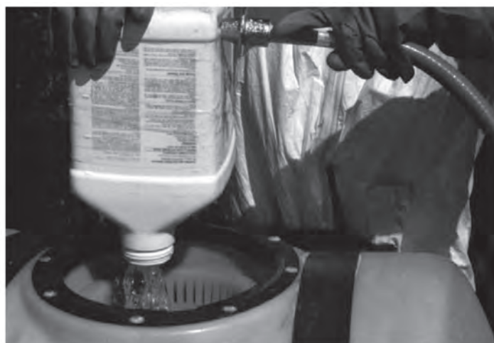
Pressure-rinsing a pesticide container.
