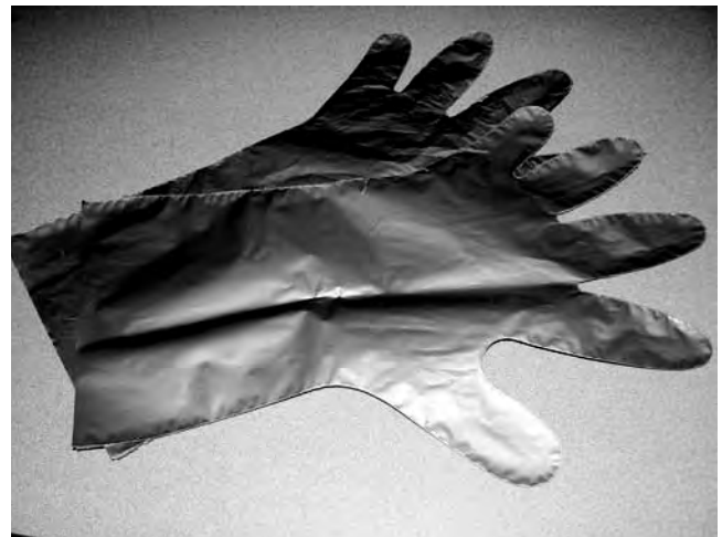
Figure 2. Example of EPA's highest rated protective glove material, barrier laminate.
