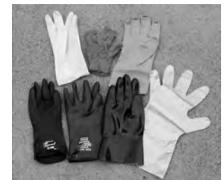
Figure 4. Chemical resistant gloves (top row, left to right): natural rubber, disposable nitrile, reusable nitrile and (bottom row, left to right) neoprene, butyl rubber, Viton, and barrier laminate.
