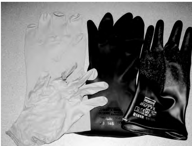
Figure 1. Examples of recommended gloves: nitrile (reusable and disposable), neoprene, and butyl rubber.
