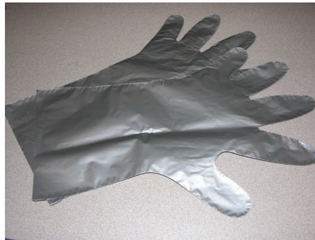
Figure 2. Example of EPA's highest rated protective glove material, barrier laminate.
