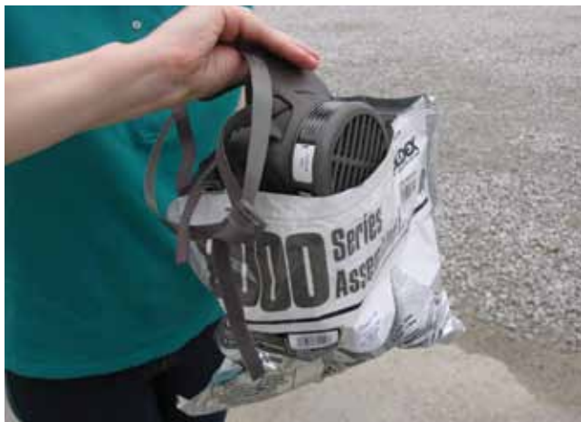
Figure 6. Store your respirator in its original packaging or a resealable zipper storage bag or plastic storage container.
