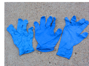
Figure 5. Disposable nitrile gloves in 4, 8, and 12 mil weights.
