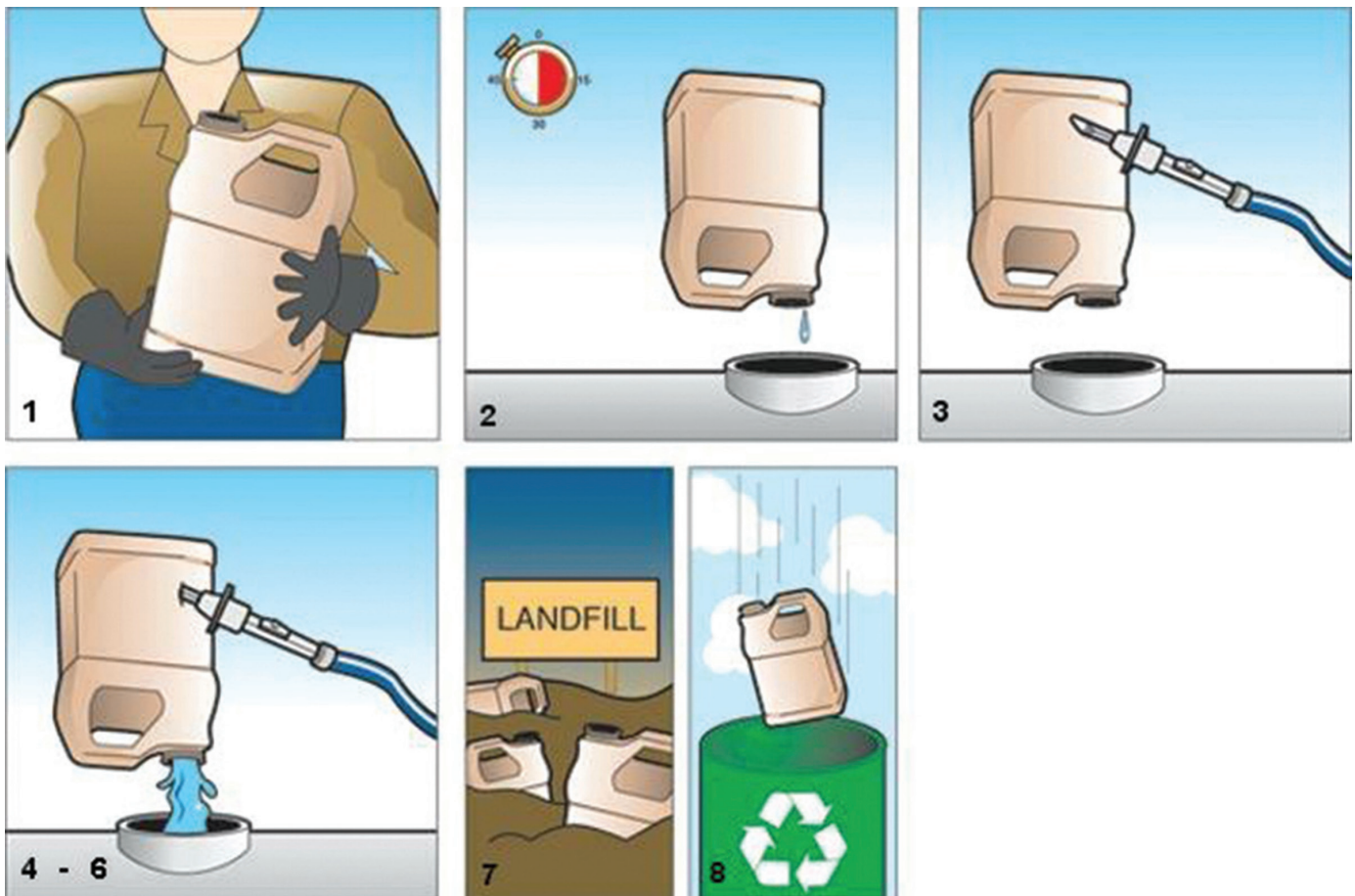
Figure 2. Pressure-rinsing procedure for plastic pesticide containers. Used with permission from Fred Whitford, Purdue University. Scott Dallas and John Metzinger, illustrators.
