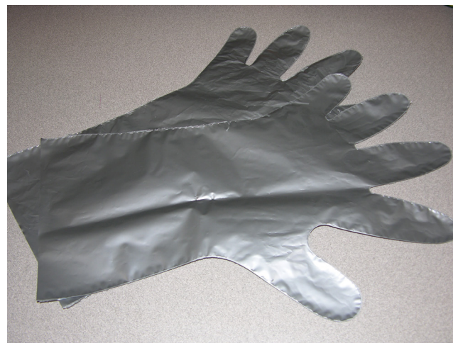
Figure 2. Example of EPA’s highest rated protective glove material, barrier laminate. Photo: University of Nebraska–Lincoln.
