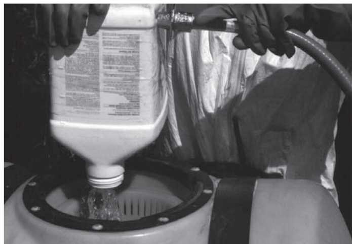
Pressure-rinsing a pesticide container.
