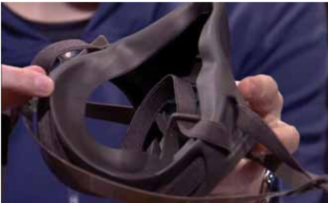
Figure 7. After each use and before storing your respirator, the faceplate should be washed with soapy water, hung to dry, and checked for wear or damage.
