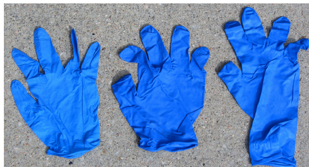
Figure 3. Disposable nitrile gloves in 4-, 8- and 12-mil weights. Photo: University of Nebraska–Lincoln.
