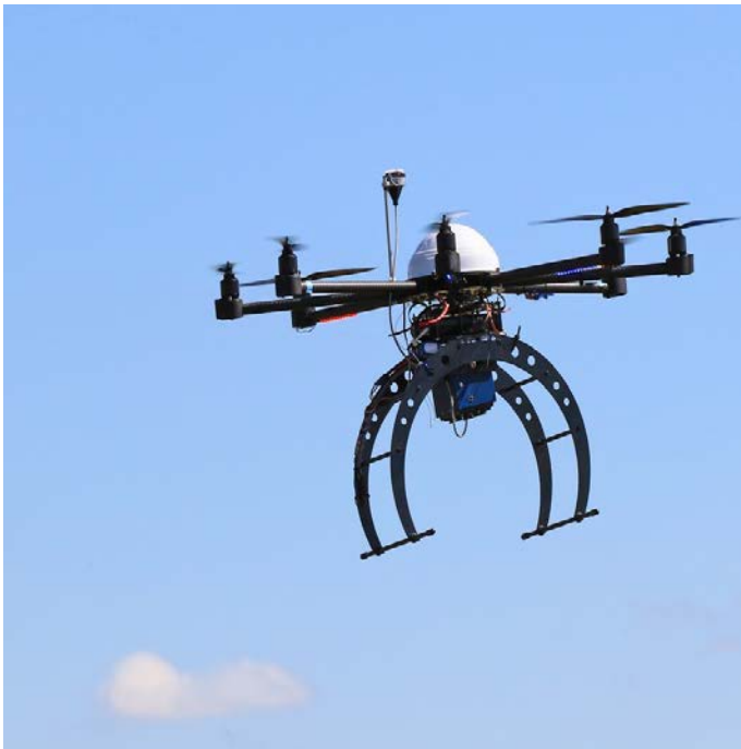
Figure 3. Multirotor UAS (Octocopter XL) with five band Tetracam MCA multispectral sensor, with incoming radiometer correction.
