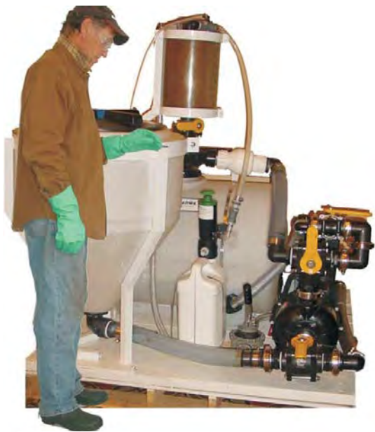
Figure 8. Because an enclosed system reduces the risk of pesticide exposure, the PPE requirements may be reduced. GoatThroat Pumps photo.
