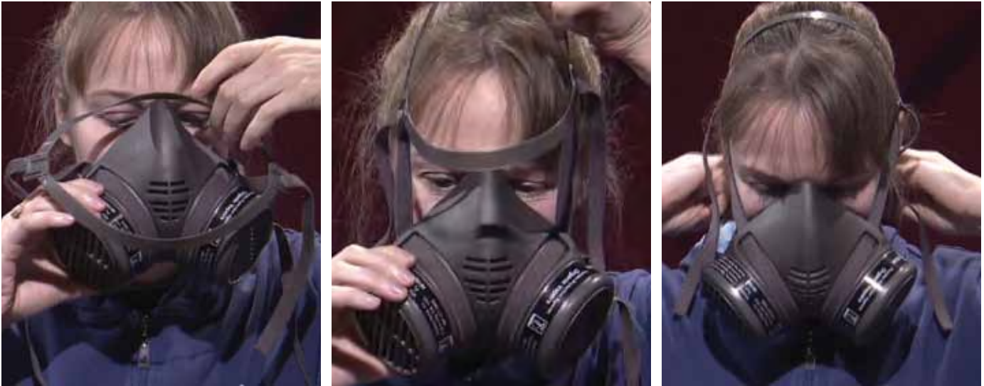
Figure 2. Adjusting a respirator step-by-step: 1. Place on face. 2. Adjust halo. 3. Adjust neck straps.
