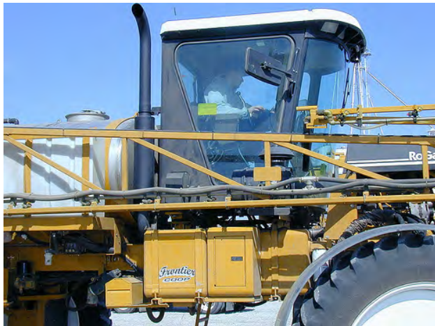
Figure 9. In some situations, PPE requirements may be reduced when a handler is in an enclosed cab. UNL photo.
