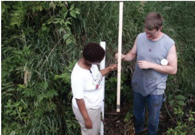
Above: Martha Mamo and Nathan Mueller observe the peak stream flow recorded by a crest gauge; granulated cork sticks to the wood inside the pVC pipe.
