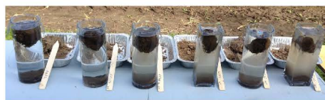
Figure 1. Slake test proxy for water stable aggregates. Left to right: Alfalfa, CCSW(rc)-NT, CCSW(rc)-CT, CCCC-CT, CCSS-NT, and CCSS-CT. NT=No-till, CT=Conventional till, C=corn, S=soybean, W=wheat, rc=red clover. Photo credit: Bill Deen, Univ. of Guelph
