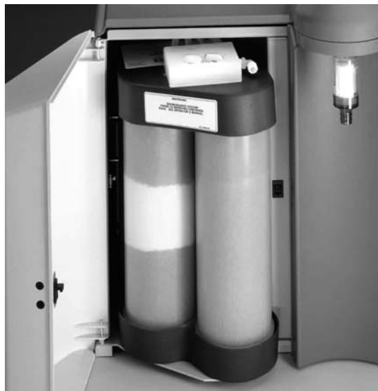
Figure 12-1. Cartridge Pack Replacement
