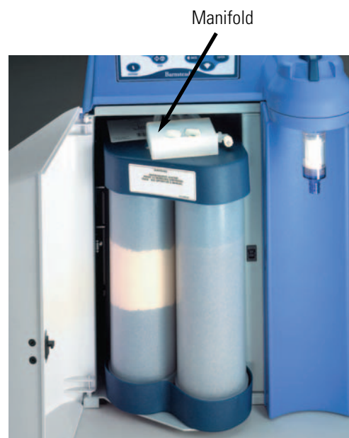
Figure 7-1. Cartridge Pack Installation
