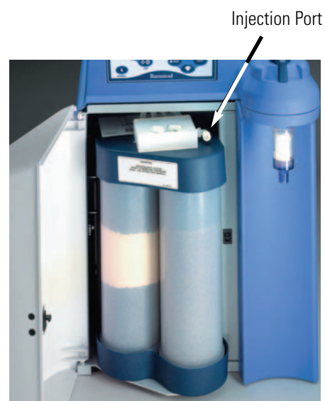
Figure 7-2. Injecting Cleaning Solution
