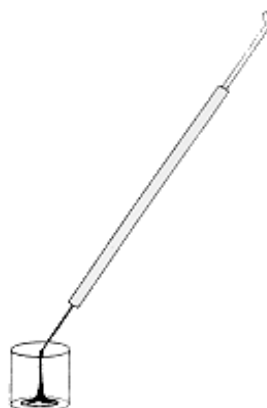
Figure 69. Introduction of a viscous sample into the container
