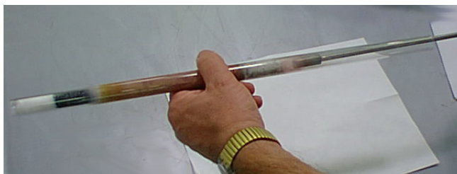
Figure 137. Removing the Filling Material from a Quartz Reactor
