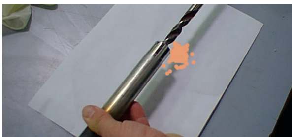
Figure 140. Collection of the Filling Material Removed from a Special Steel Reactor
