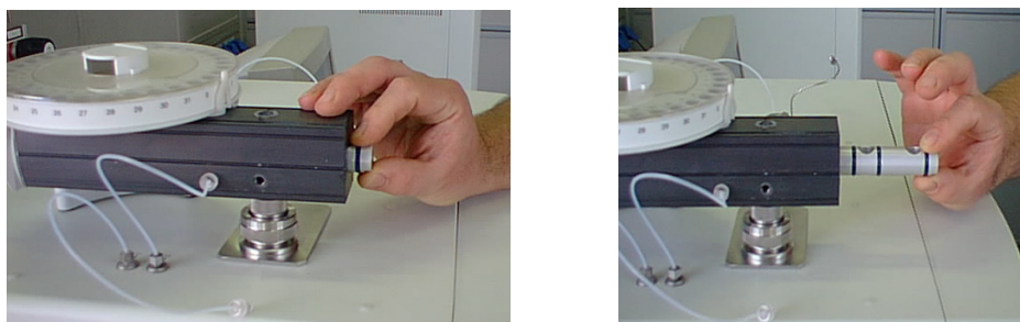
Figure 156. Removal of the shaft
