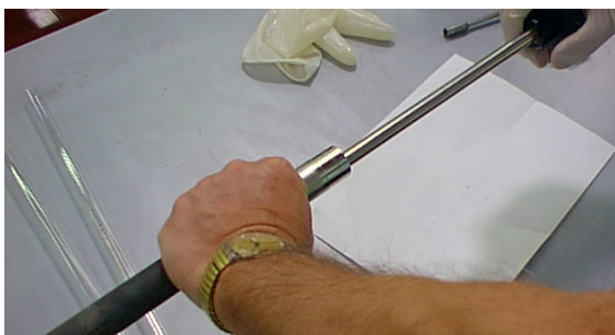
Figure 139. Removal of the Filling Material from a Special Steel Reactor
