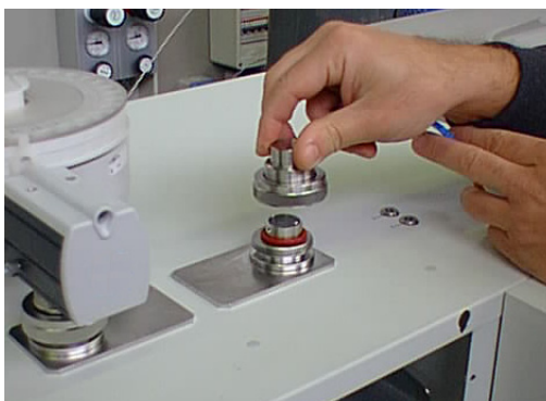
Figure 50. Mounting the fixing nut on the right furnace
