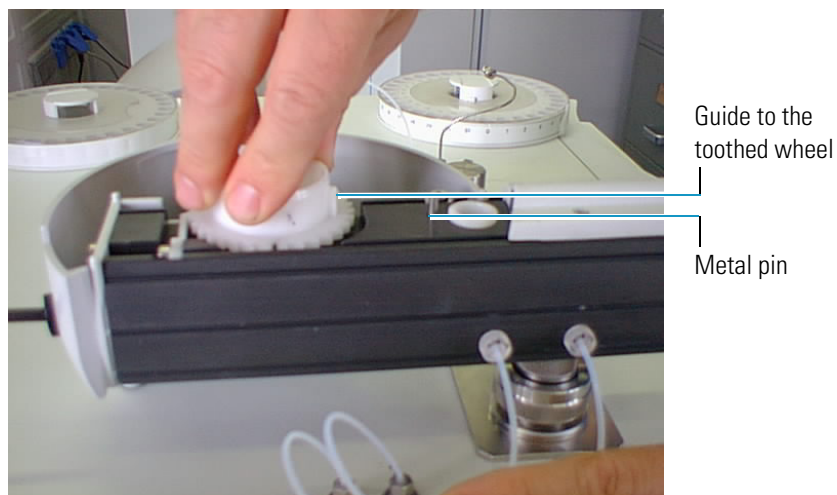
Figure 152. Alignment of the Toothed Wheel
