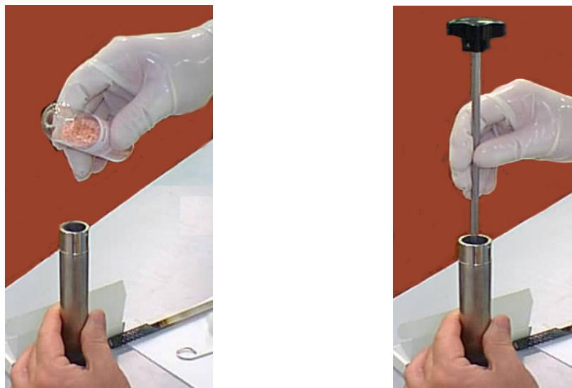
Figure 31. Filling of the special steel reactor and compression of materials
