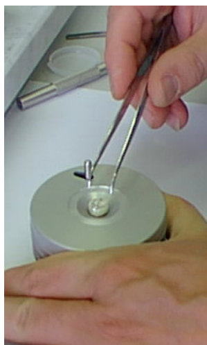
Figure 63. Removal of the closed container and cleaning of the contact surface
