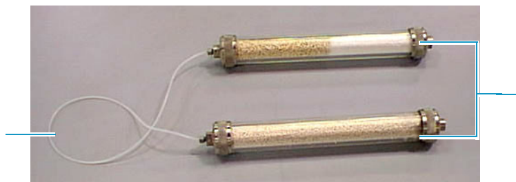
Figure 53. Connection of two filters in series
