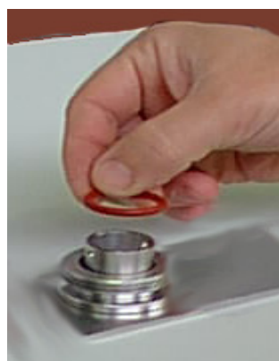
Figure 56. Removal of the steel reactor o-ring
