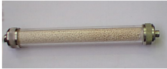
Figure 38. Result of the filling of a large adsorption filter and of a small one
