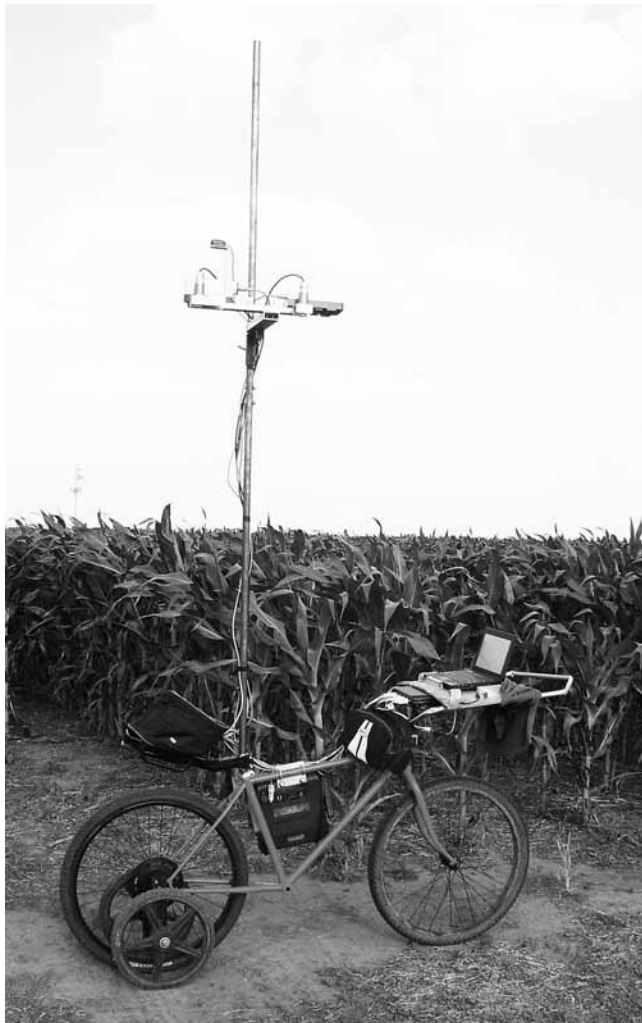
Fig. 1. Platform for data acquisition (bicycle equipped with two optical sensors, DGPS, laptop computer, and batteries).
