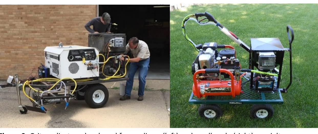
Figure 2. Grit applicators developed for medium- (left) and small-scale (right) specialty crop production. The two-nozzle applicator would retail for approximately \$12,500, compared to \$3,500 for the hand-held, single-nozzle applicator.
