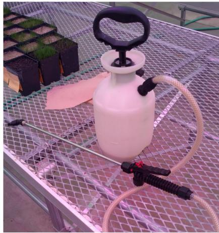
Figure 2. The sprayer used to apply bio-based film solutions. Rates were calibrated using a graduated cylinder and a stopwatch.
