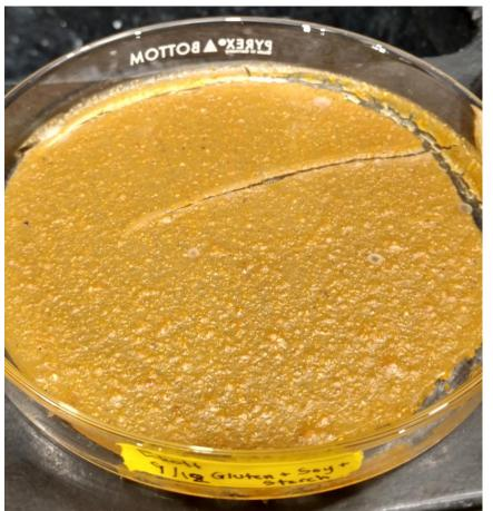
Figure 1. The 5 ingredient solution. This film had the fewest cracks among 9 solutions prepared in petri dishes.
