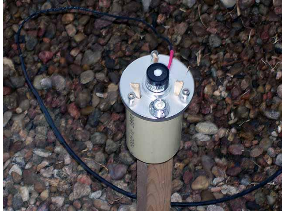
Figure 1. Close-up of LiCor PAR Sensors. One incident and one reflective PAR over red plastic.
