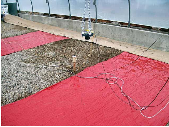
Figure 1. Close-up of LiCor PAR Sensors. One incident and one reflective PAR over red plastic.
