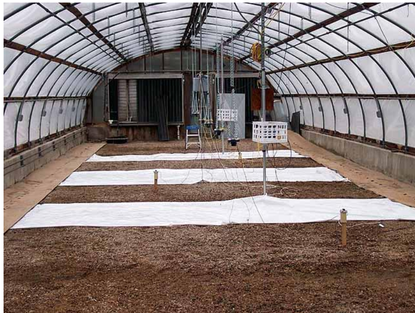
Figure 2. Reflective Mulch and Surface temperature Study with 6-mil white plastic.
