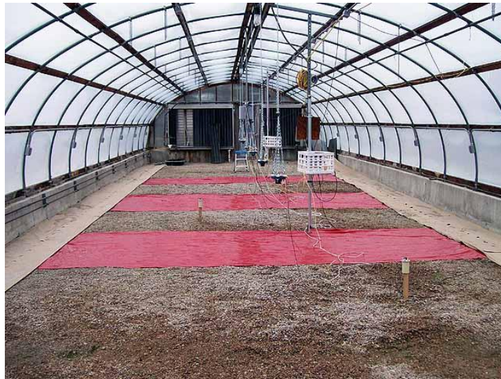
Figure 3. Reflective Mulch and Surface temperature Study with 4-mil red plastic.
