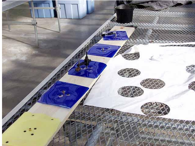
Figure 8. Cutter board system for producing holes in the plastic reflective mulch fabric.
