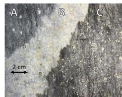
**Figure 4.** A bird's eye view of a deconstructed piece of PLA/soy biomulch including: A) spunbond PLA fibers in the bottom layer; B) meltblown PLA sheet with embedded soy in the middle layer; and C) spunbond PLA fibers in the top layer.
