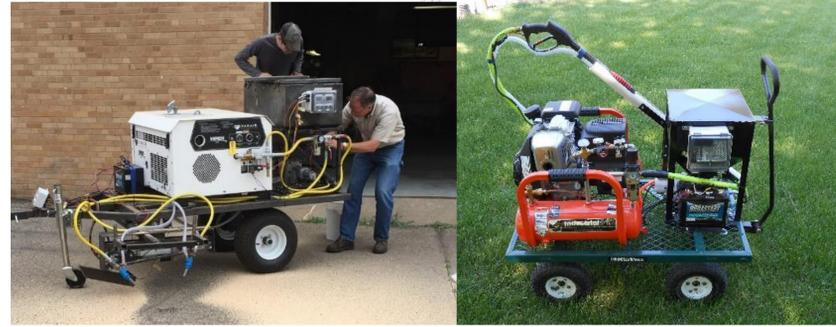
Figure 2. Grit applicators developed for medium- (left) and small-scale (right) specialty crop production. The two-nozzle applicator would retail for approximately \$12,500, compared to \$3,500 for the hand-held, single-nozzle applicator.
