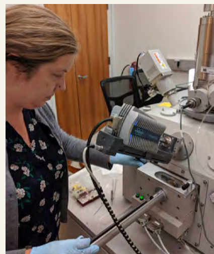
Jennifer Cooper analyzes biochar surface characteristics using scanning electron microscopy.
