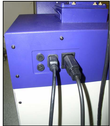
Left cable: Main Power cable; Right: Transilluminator jumper cable
