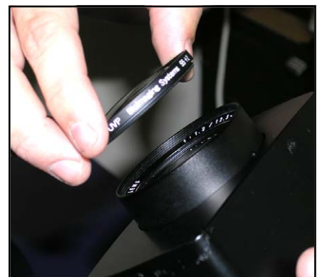
Screw the step-up ring and dioptr onto the lens
