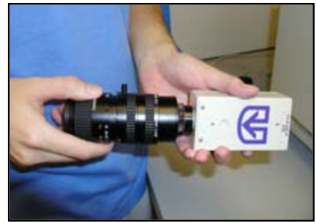
Screw the lens onto the Camera
