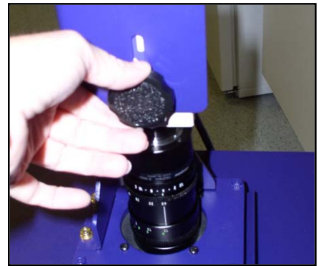
Connect the Camera to the Bracket
