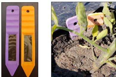
Figures 3 & 4. Anion and cation pair of PRS probes to measure plant available  $\text{NO}_3\text{-N}$  and  $\text{NH}_4\text{-N}$ . (New and buried pairs, respectively.)
