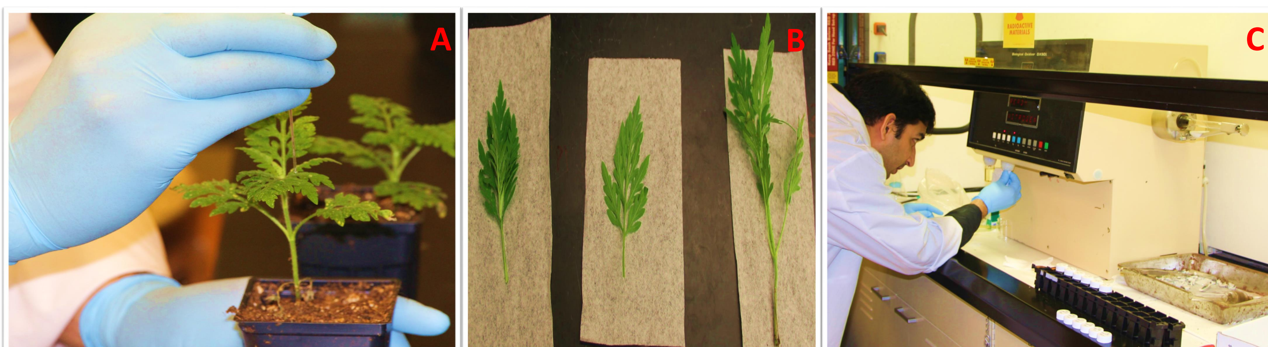
Figure 1. Procedure of the absorption and translocation study. (A). Applying 14 C labelled herbicides; (B) Treated plant cut into sections (tissues ATL, TL, tissues BTL); (C) Burning of the oven-dried samples in a biological oxidizer to recover applied radioactivity as 14 C labelled CO 2 from different plant sections; (D) Liquid scintillation spectrometer used to quantify 14 C labelled herbicide recovered from different plant section during burning.
