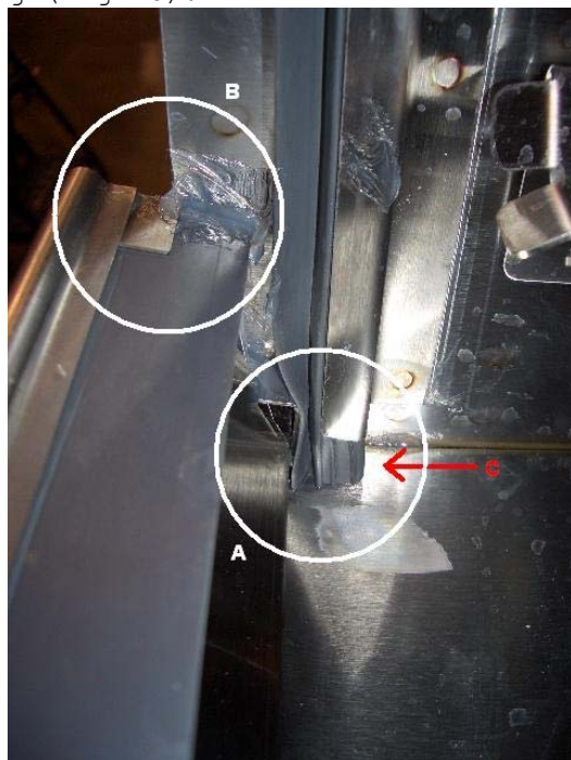
Figure 33: Bottom front left corner of washer tank. With the door off you can find the clips and RTV application used to hold the gaskets into place. Circle A: There may or may not be a clip holding the door gasket in place. If there is, this must be taken out to remove the damaged gasket.
