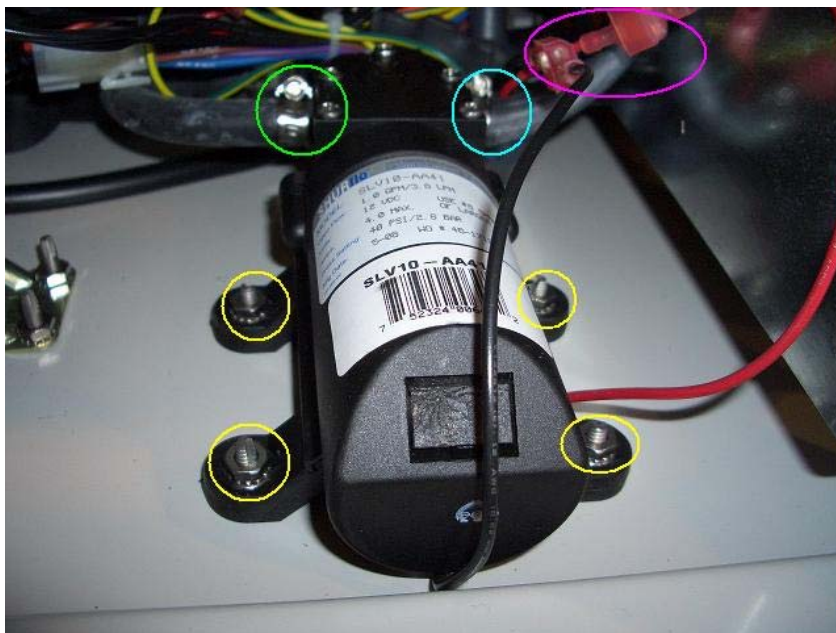
Figure 18 Left: DI/Pure Water Pump. The Pure water pump is located in the Front Left of the machines base. The Yellow Circles indicate the four nuts that mount the DI Pump to the base of the unit.
