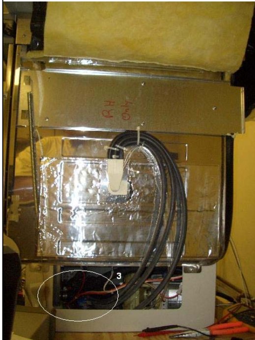
Figure 5: (left) Front view of glassware washer. Circle "4" indicates location of where the Drain Pump can be found (see Figure 4) Figure 6: (right) Side view of glassware washer. Circle "3" indicates location of where the Drain Valve & Pump can be easily seen/found (see Figures 3 & 4).
