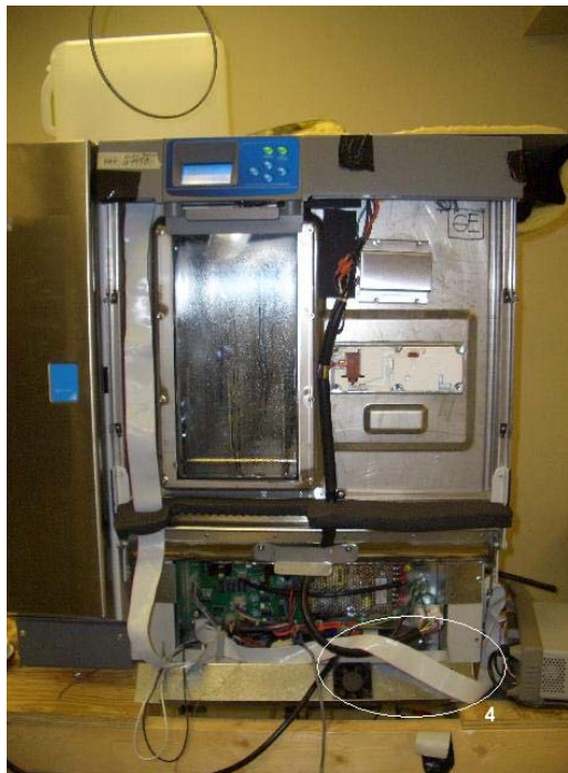
Figure 5: (left) Front view of glassware washer. Circle "4" indicates location of where the Drain Pump can be found (see Figure 4) Figure 6: (right) Side view of glassware washer. Circle "3" indicates location of where the Drain Valve & Pump can be easily seen/found (see Figures 3 & 4).
