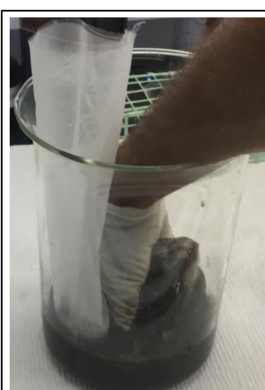
Figure 3: CE was prepared by kneading 100g dry equivalent mass compost in a 450um nylon mesh bag submerged in 1000mL total water.
