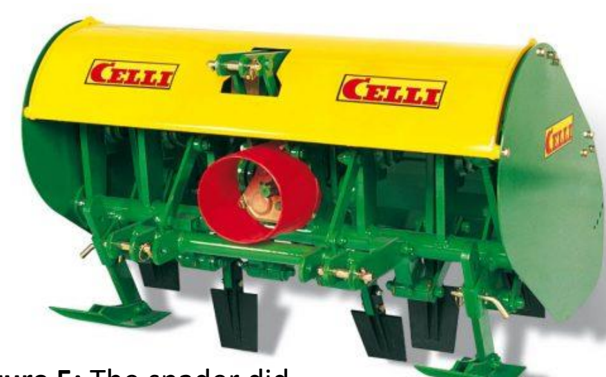
Figure 5: The spader did not get tangled with either PLA-W or BP mulch, as rototillers have been reported to do.
