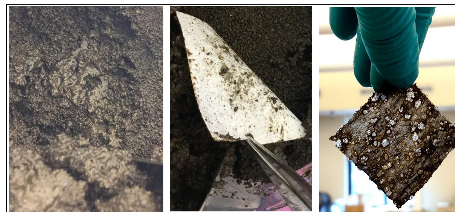
Figure 1: Total degradation of PA (left). No mass loss of PLA, slight hydrophobicity visible (center). Cleaned PLA-S showing near complete loss of soy particles with only PLA remaining.
