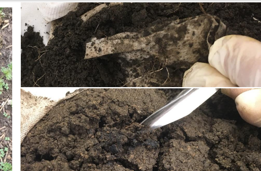
Figure 7: Top: one year after burial PLA-W is in-tact, bottom BP was visible but too deteriorated to recover. Final samples to be recovered Fall 2019.
