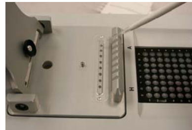
Loading samples on position A when operating within the Single Sample Mode.
