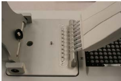
Loading samples when operating within the 8 Sample Mode.
