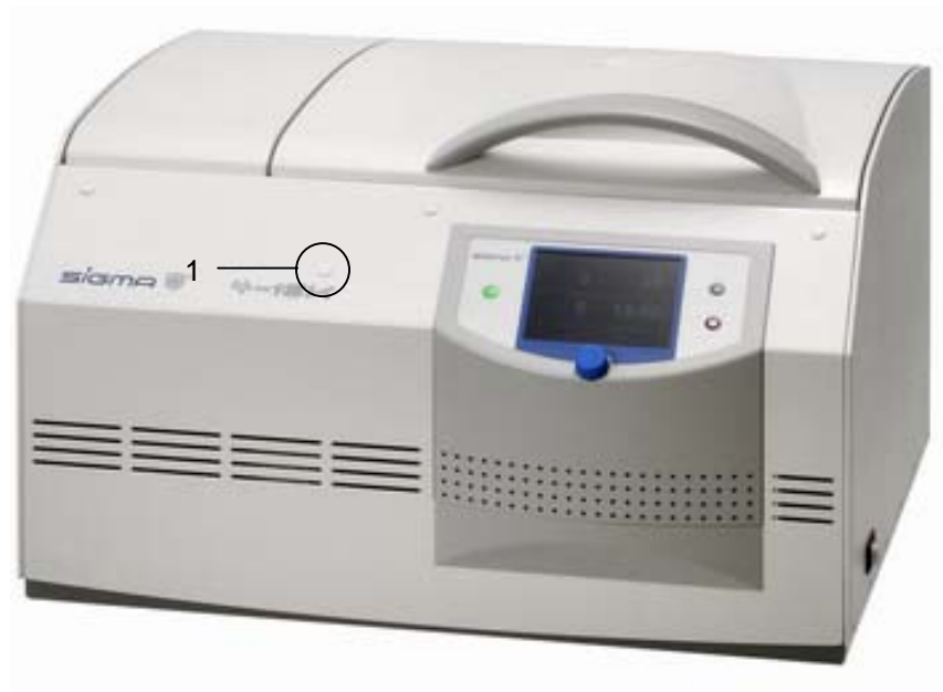
Fig. 7.2: Position of the opening for the emergency lid release
