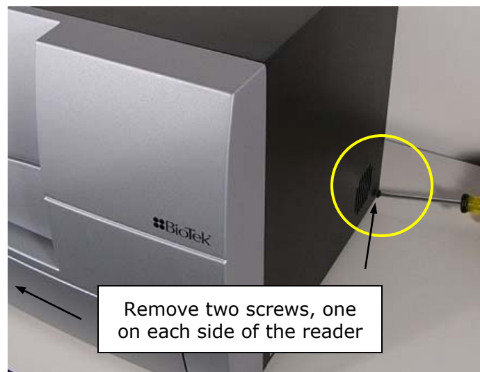
Figure 2: Removing the two side screws.
