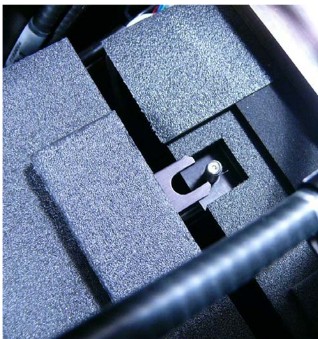
Figure 54: Incubator housing "fork" in the correct position
