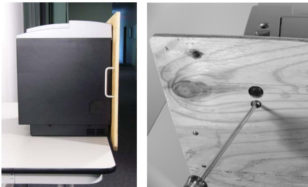
Figure 1: The reader on its back with the shipping panel attached to the bottom (left), and removing the screws (right).
