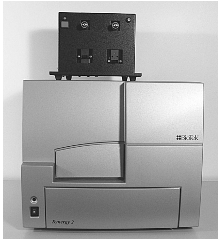
Figure 11: The dispense module on top of the reader.
