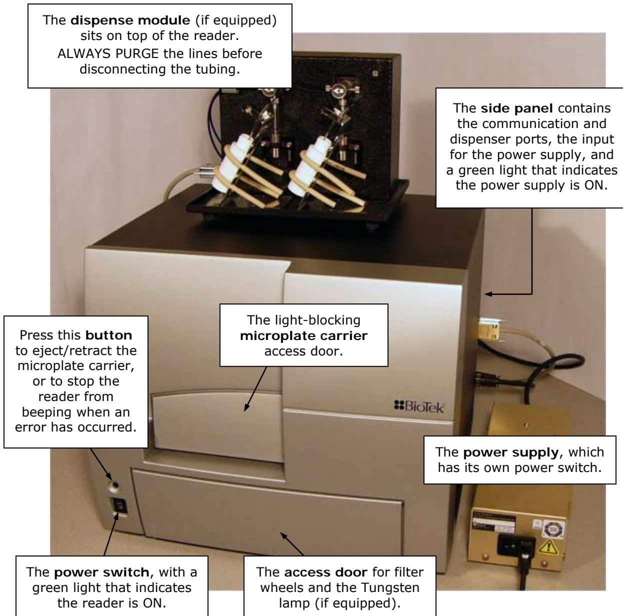
Figure 18: Identifying the main external components
