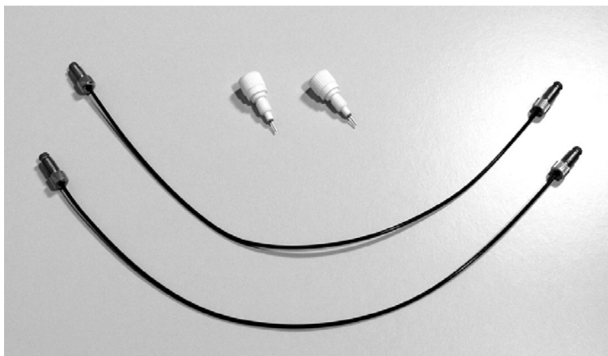
Figure 46: Injector heads and internal dispense tubes
