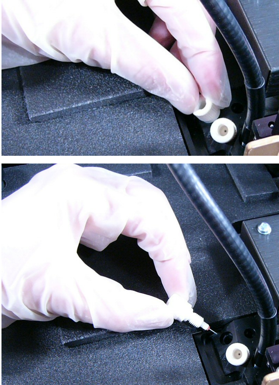
Figure 45: Remove the injector heads
