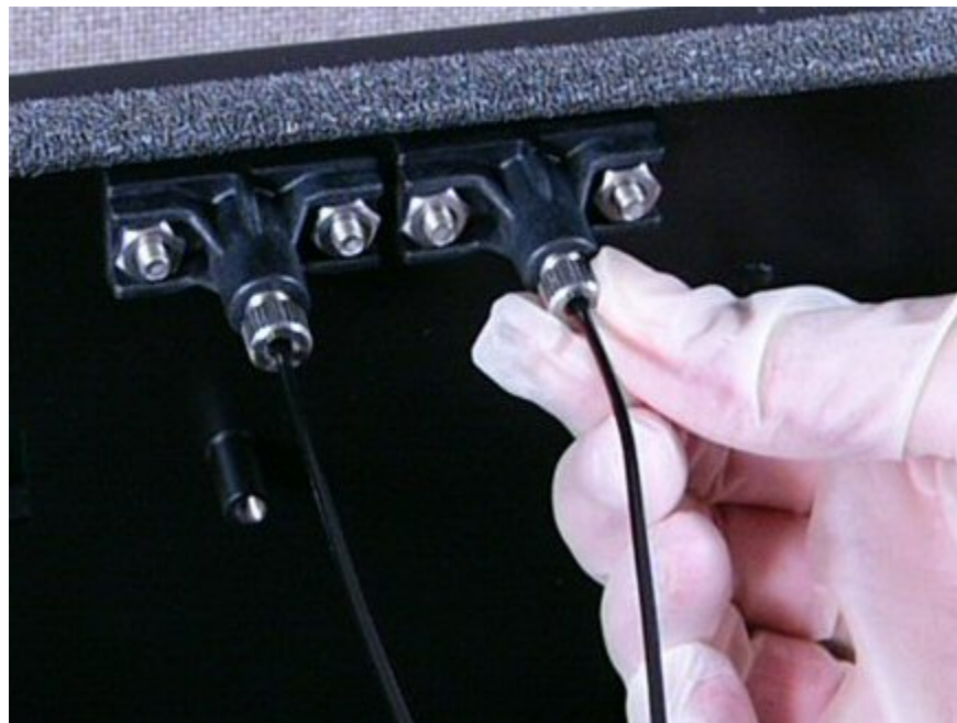
Figure 43: Disconnect the dispense tubes from the back wall
