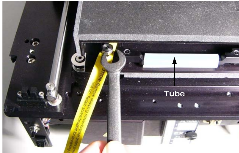
Figure 5: Remove microplate carrier shipping screw and tube.
