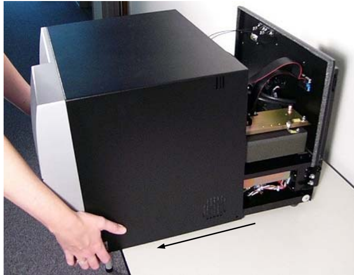
Figure 3: Sliding off the shroud.
