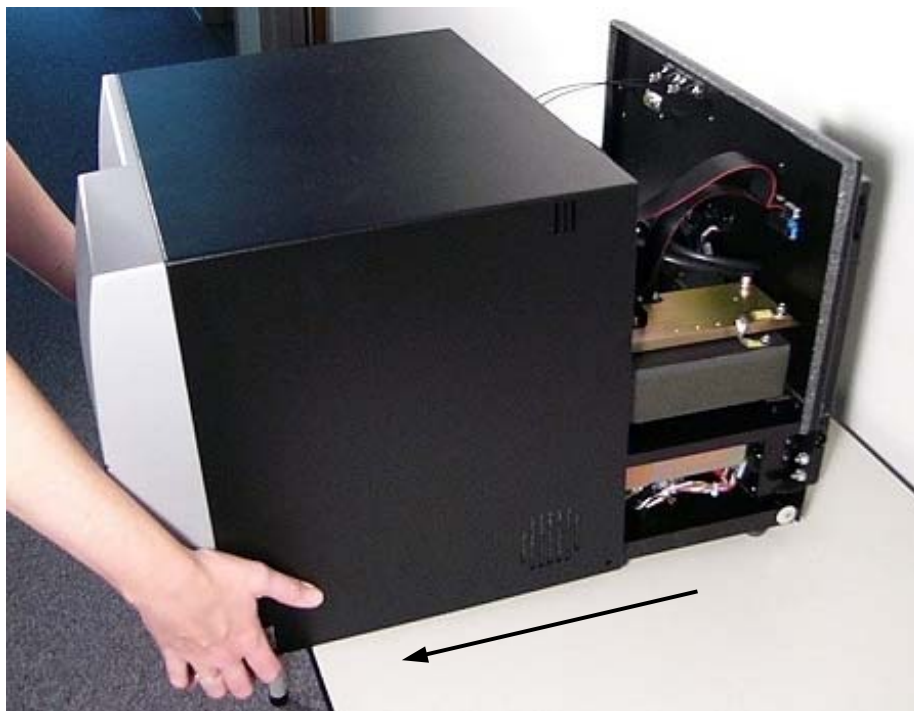
Figure 41: Removing the reader's shroud
