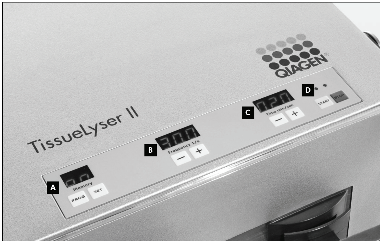
Figure 3. Keypad of the TissueLyser II. A "Memory" display, with "PROG" and "SET" keys for storing disruption parameters. B "Frequency 1/s" display, with "-" and "+" keys for adjusting oscillation frequency. C "Time min/sec" display, with "-" and "+" keys for adjusting disruption time. D "START" and "STOP" keys for starting and stopping operation of the TissueLyser II.
