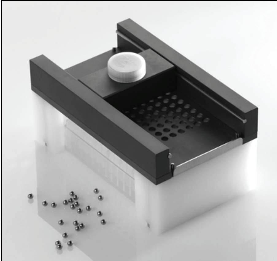
Figure 9. TissueLyser Bead Dispenser, 96-Well. The dispenser dispenses 96 beads into a rack of collection microtubes.
