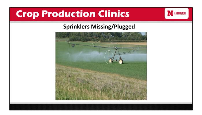
Uniformity is critical during a chemigation application. Check system for proper nozzle operation. Get out nozzle chart from the manufacturer to make sure the correct nozzle is in the correct location.
