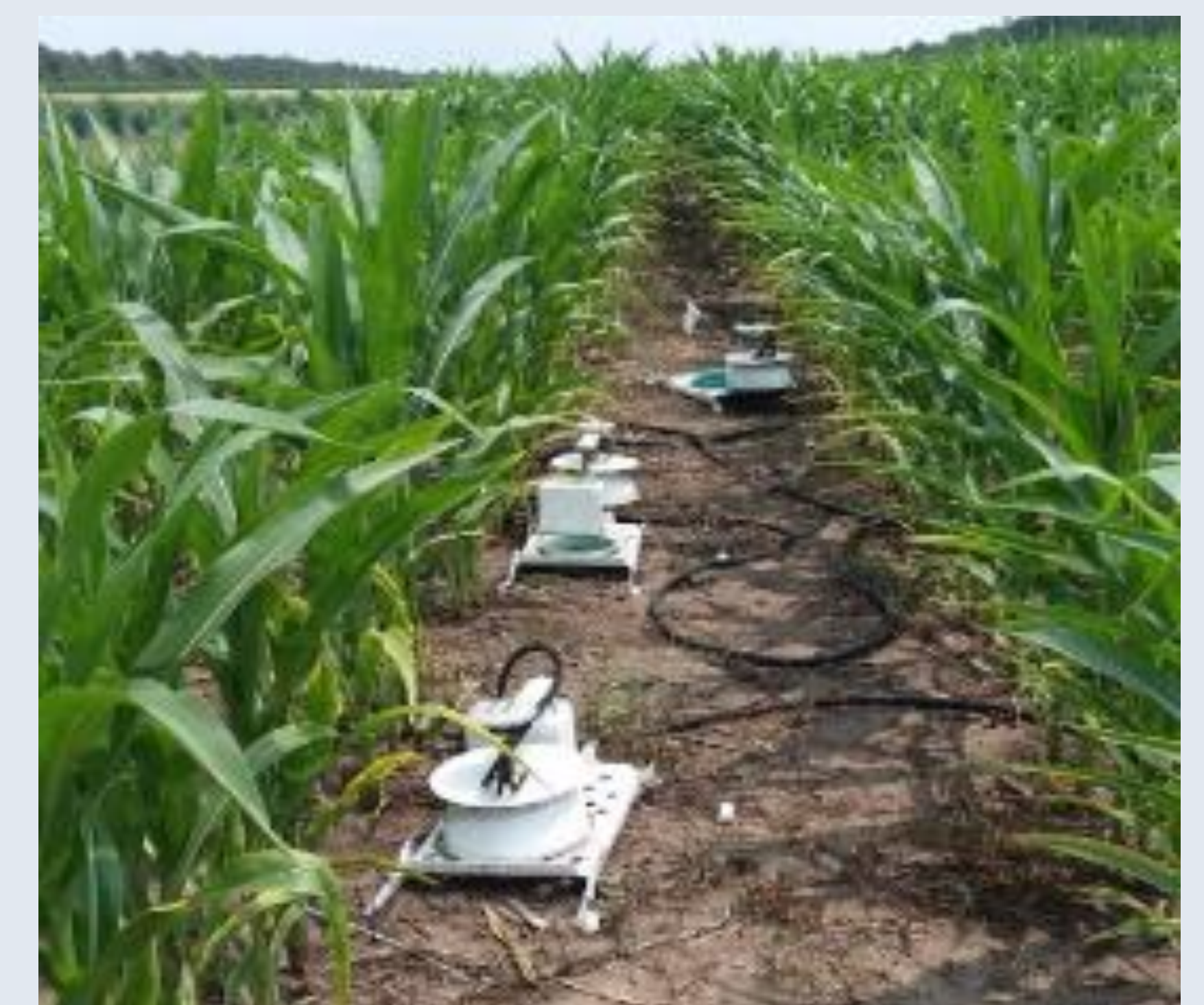
Figure 5. Open LI-COR LI-8100-104 long-term opaque chambers connected to the Picarro® Instrument
